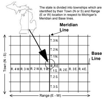
A township is normally a quadrangle approximately 6 miles on a side which contains thirty-six (36) sections. As shown below in some townships corrections for the earth's curvature will show up on it's northern and western boundary lines. Also, note the way in which sections are numbered within a township.
